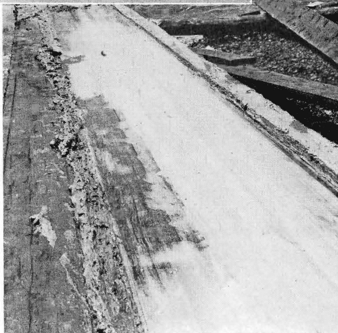
Unable to support the weight of a large ship the greases in the photo on the left squeezed out excessively, permitting wood to wood contact between the ways which might seriously have interfered with the launching. The greases in the right photo also squeezed out under the pressure but maintained a sturdy film of lubrication between the ways necessary for safety.
