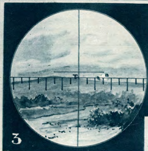
3 DEFLECTION GRATICULES OF A PRISM BINOCULAR. TARGET MARKED T. SHELL BURST B.
