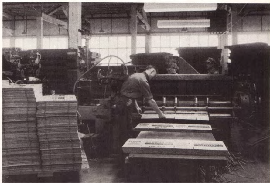
Langston two-color printer-slotter built for speed production of small and medium size boxes.
