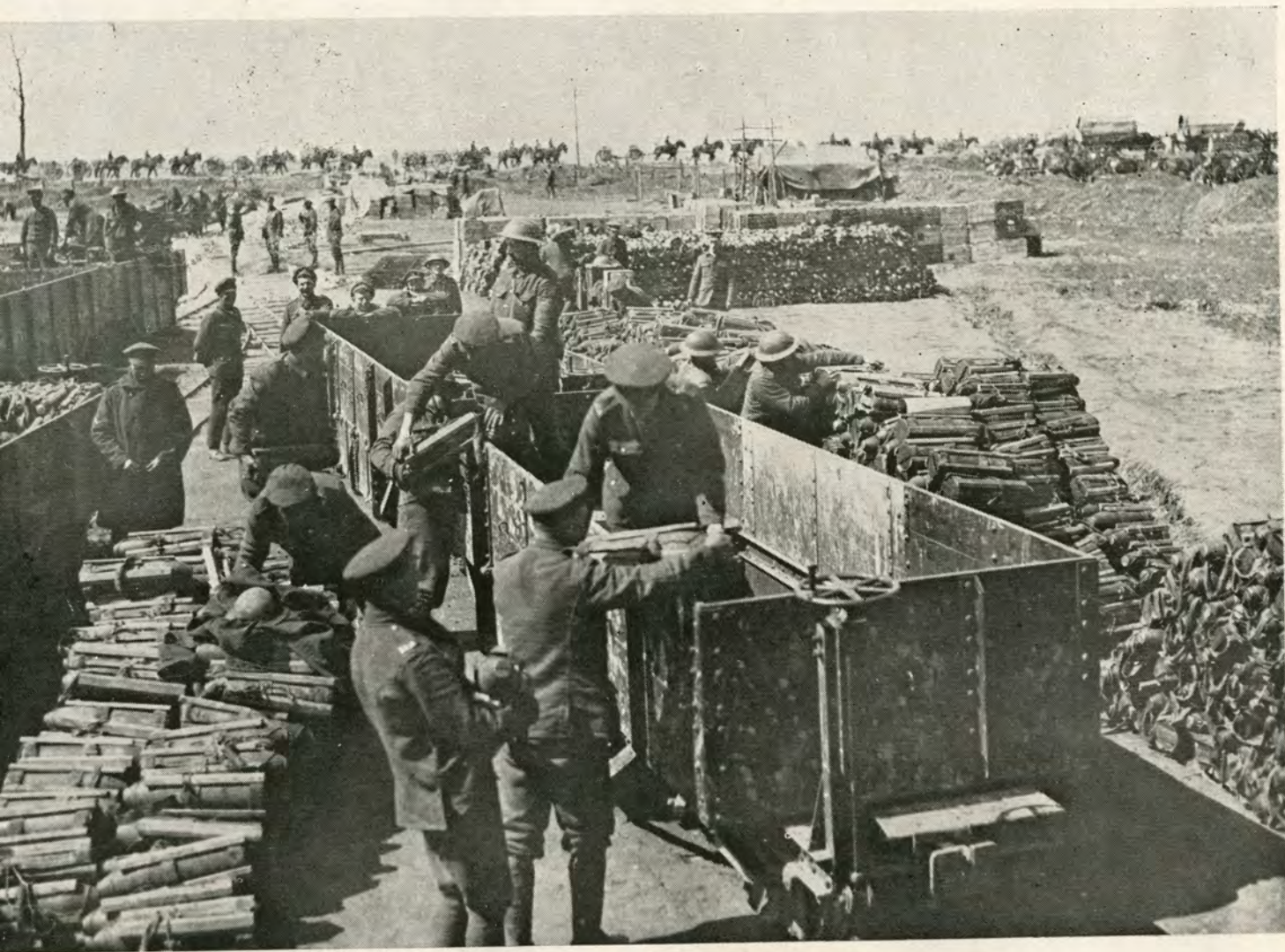
AN AMMUNITION LOADING POINT ON THE NARROW GAUGE RAILWAY. Note how each shell is packed in wood to protect it from damage.
