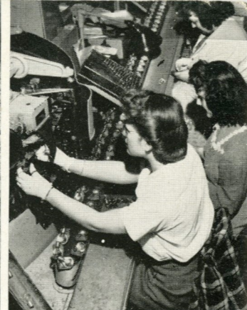
THE ARMY JEEP, left, like armoured cars, tanks, army trucks, etc., uses headlamp bulbs exactly the same as those in passenger cars. Betty Durkin, right, is basing these prefocused 2-filament lamps. Also taking an important part in this operation are Cornelia Bailey and Connie Hall.
