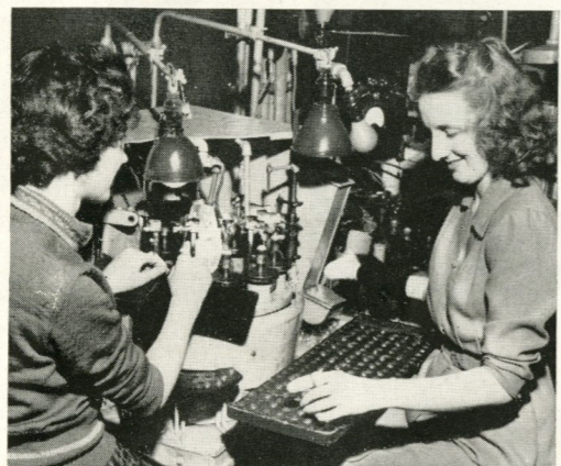
MAKING FLASHLIGHT LAMPS are Betty Mackeridge, left, centering filament, and Vera Lawler, operating butt sealing machine. It turns out approximately 1000 lamps hourly. Millions of these tiny lamps have been ordered for the Armed Forces. Queer patterns, right, are made by airman signalling incoming plane with flashlights.
