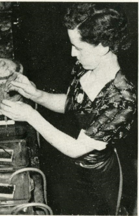
LAMP FILAMENTS ARE GIVEN AN ACID BATH, left, by Muriel Wood, WD-2. Acid eats away steel core around which filament is wound. Right, Allied planes require many types of lamps, the filament of which is not the least important.
