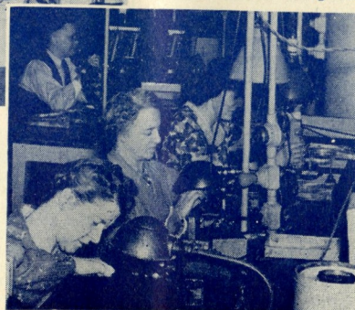
ABOVE—Workers are using the edge-grinding machines which shape the lens as required by the prescription and grind the edges smooth.
