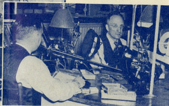
ABOVE—The two machines (referred to above) used in checking lenses are "lensometers" and "axisfinders". The former is used to check the accuracy of the various curves. The axis finders are used for marking the lenses according to the prescription.
