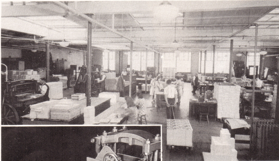
A section of the Bindery where the finishing operations, such as trimming, folding, binding, die cutting and inspecting are completed.
