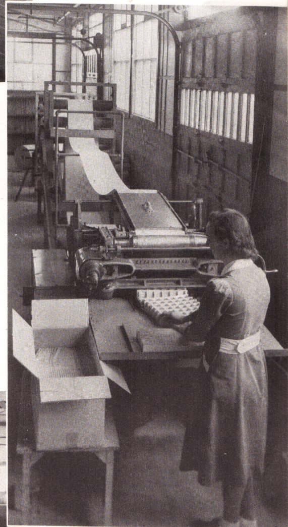
Patented Self-Locking Egg Filler Machine. Completes manufacture of all sizes in one operation.
