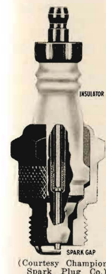
Fig. 9.—Showing the parts of a well made spark plug.
